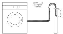
When discharging into a standpipe ensure that the top of the standpipe is no more than 90 cm (35.4") and no less than 60 cm (23.6") above floor level.
